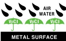
*Bull Frog®* VpCl<sup>®</sup> bond with metal surfaces to form a protective 'Molecular Umbrella,' sealing out air and moisture that cause rust and corrosion.
